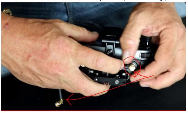
20. Place the antenna pins into the holes on the antenna bracket.
