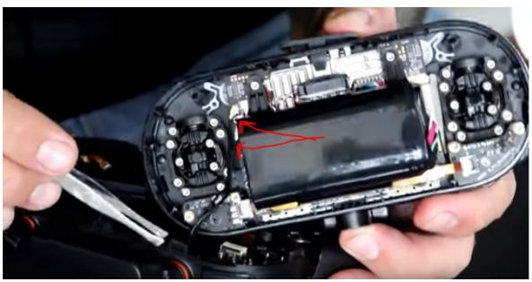
7. Gently pull off both of the the gold colored connectors, so you can just work with the other side of the controller.
